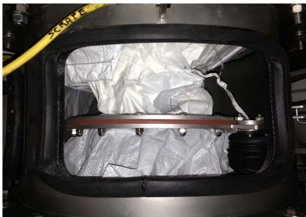
5. Untie bulk bag's discharge spout knot to let product flow freely
