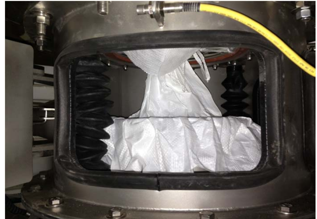
2. Spread the bulk bag's discharge spout over sealing stub
