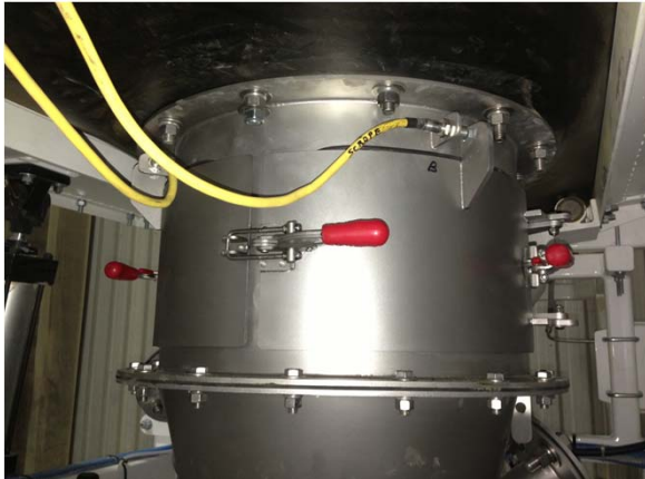
1. Unlatch 3x toggle clamps to open both access doors
