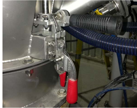
4. Lock sealing device with both toggle clamps
